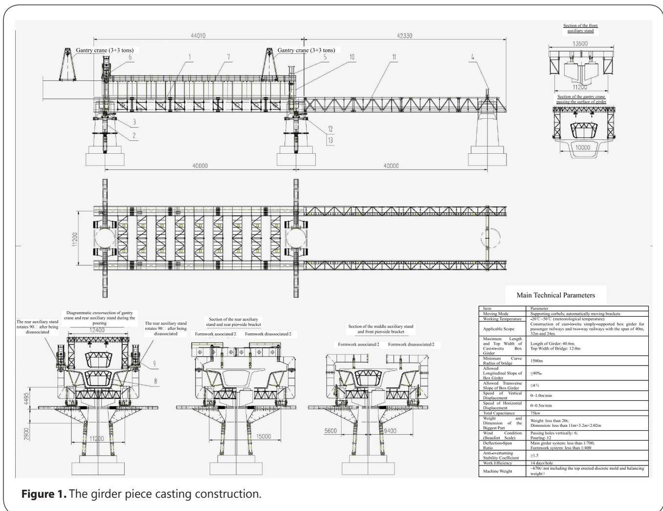
Figure 1. The girder piece casting construction.
