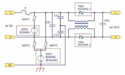
Figure 2 The main electrical protection measures
