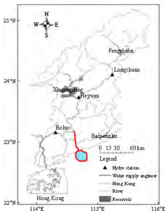
Figure 12. Dong River Basin and water diversion from Dong River to the proposed coastal reservoir (red line and oval).
