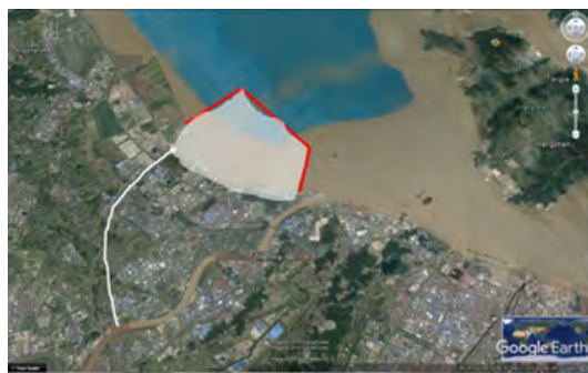
Figure 3. A proposed coastal reservoir for Ningbo and a 10 km long canal to be built to divert water with good quality to the coastal reservoir in flood periods.
