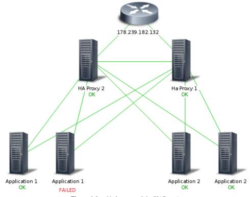
Figure 6. Load balancer module (HAProxy).
