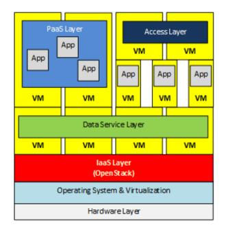
Figure 5. Decoupling the application stack.
