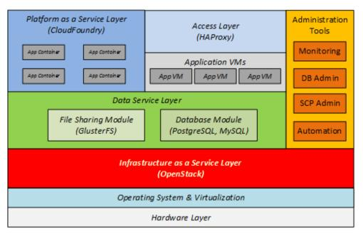
Figure 2. Storm Clouds Platform architecture.
