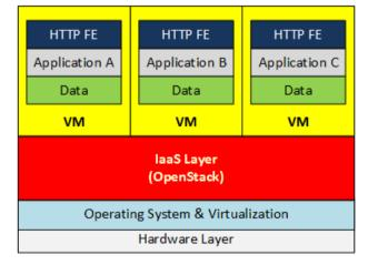
Figure 4. Deploying applications on IaaS.
