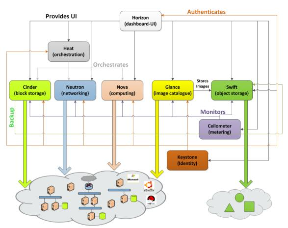
Figure 3. OpenStack logical architecture.
