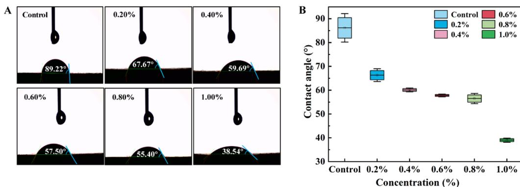
**Figure 7.** Determination of contact angle of R1-2 solutions at different concentrations over the hydrophobic surface. (A) Images of contact angles measured with a HS-150A pendant drop apparatus on core slice in aged crude oil. (B) Changes in wetting angle of core slices treated with different concentrations of surface.
