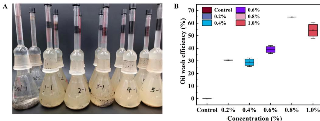
**Figure 8.** Efficiency of oil washing of biosurfactants produced by R1-2. (A) Images of the amount of oil washed out by different concentrations of BS. From left to right, represent the control, 0.2%, 0.4%, 0.6%, 0.8% and 1.0% experimental group, respectively. (B) Variation of wash out the oil content with surfactant additions.
