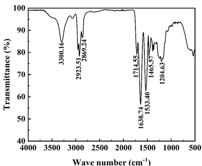
**Figure 4.** FT-IR spectrum of the purified biosurfactant produced from the *Bacillus Subtilis* R1-2. FT-IR spectrum analysis shows the spectrum of purified bioemulsifier at 400-4000 wave numbers ( $\text{cm}^{-1}$ )
