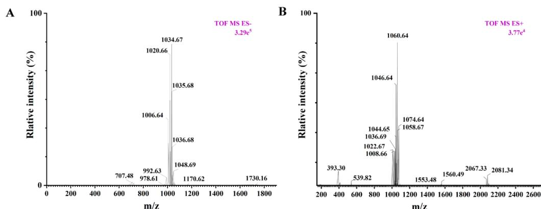
**Figure 3.** Mass spectrometry of biosurfactants produced by *Bacillus Subtilis* R1-2. (A) Negative ionization mass spectrometry. (B) Positive ionization mass spectrometry.
