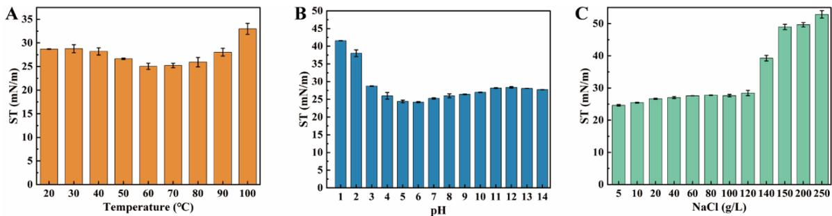
**Figure 6.** Surface tension of biosurfactant after the tolerance test upon different physicochemical conditions. (A) temperatures. (B) pH and (C) NaCl concentrations.
