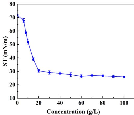
**Figure 5.** The surface tensions against the concentrations of the biosurfactant produced by the strain R1-2 in solutions.
