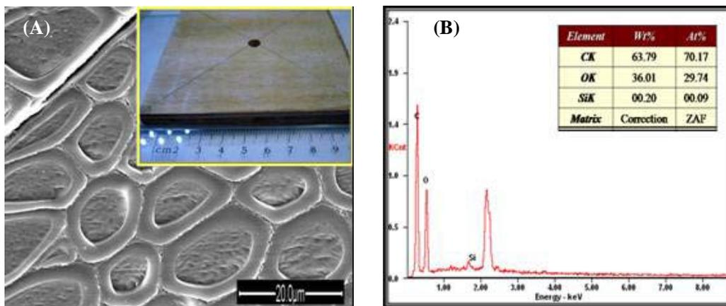
**Figure 2.** Electron microprobe analysis of wood-polymer-SiO<sub>2</sub> hybrid nanocomposite, (A) transversal face, and (B) Si elemental distribution.
