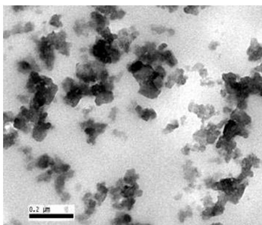
**Figure 3.** TEM morphologies of the wood-polymer-SiO<sub>2</sub> hybrid nanocomposite.
