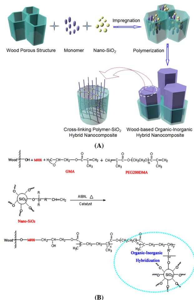
**Figure 1.** Schematic illustration to: (A) the preparation of wood-based organic-inorganic hybrid nanocomposite and (B) the mainly probable reaction mechanism.
