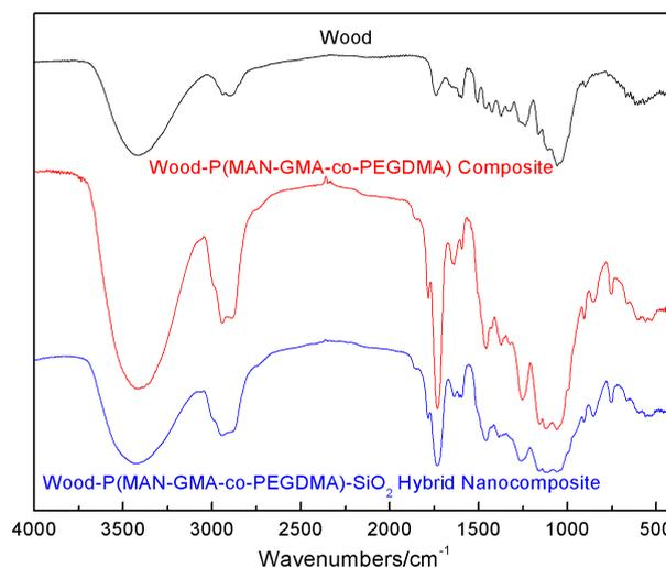
**Figure 4.** The FTIR spectra of wood, wood-polymer composite, and wood-organic-inorganic hybrid nanocomposite.
