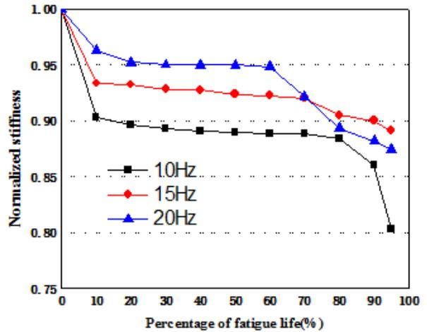
Figure 7. Stiffness degradation curves of the composite materials under three loading frequencies.
