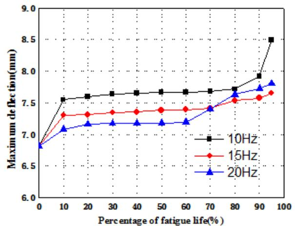
Figure 8. The deflection curves of the composite materials under three loading frequencies.
