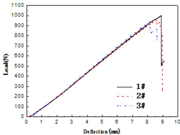
Figure 3. Quasi-static bending Load-Deflection curve.
