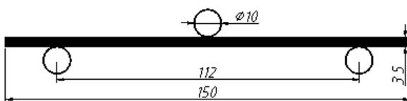
Figure 1. Sketch of three-point bending test.
