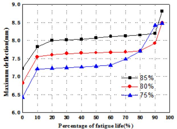
Figure 5. The deflection curves of the composite materials under three stress levels.
