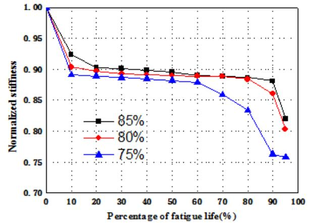
Figure 4. Stiffness degradation curves of the composite materials under three stress levels.
